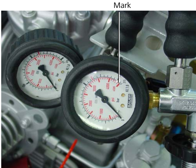
Abb. 33 Final pressure gauge
