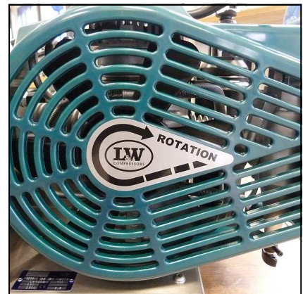
Rotation direction arrow on the fan protection cover.
