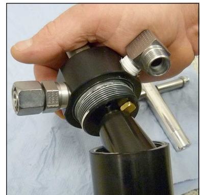
Fig. 3 - Turn off and remove separator head
