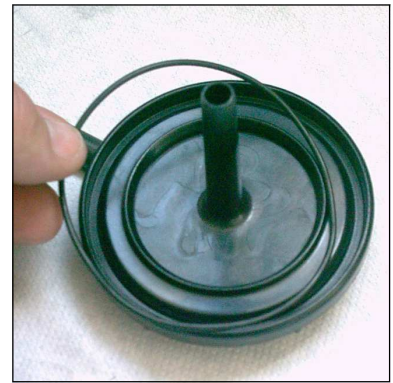
Fig. 3 - Place o-ring into the filter housing
