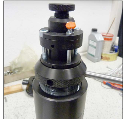
Fig. 1 - Remove/screw in filter cover
