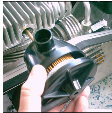
Fig. 2 - Pull out filter housing carefully
