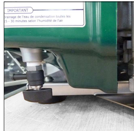
Fig. 1 - Condensate drain valve 1.stage
