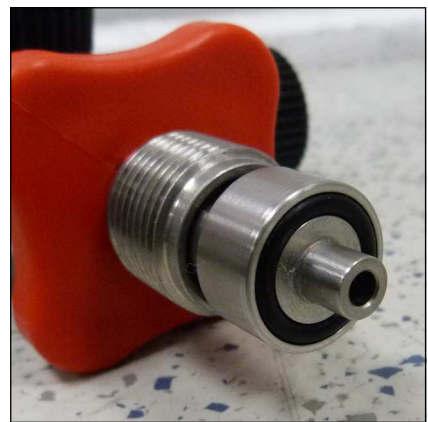
Fig. 1 - O-ring at the filling valve
