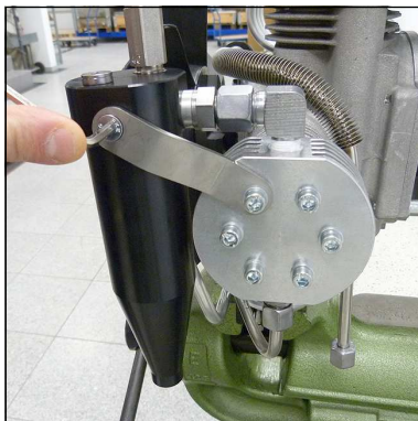
Fig. 1 - Loosen mounting screws
